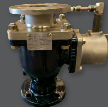
GA/FIG: 8340 4" Double Orifice Flanged ANSI 150# Ali-Bronze Air Valve c/w flanged piped outlet, coated with black epoxy.
